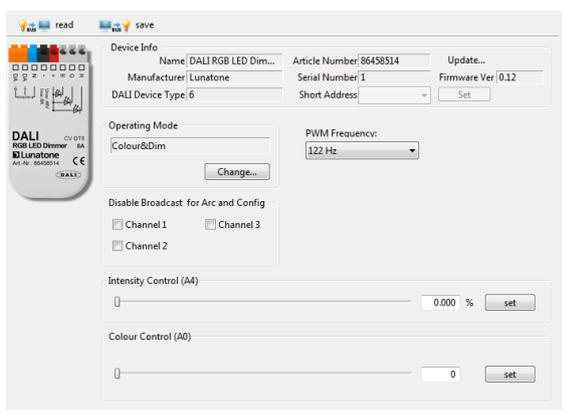
Switching between operating modes can also be done with the help of the DALI-command SET OPERATING MODE (IEC 62386-102 Ed.2). When changing the operating mode the number of used DALI-addresses can change as well and this requires a new addressing procedure. In the DALI-Cockpit this address assignment is performed automatically.
