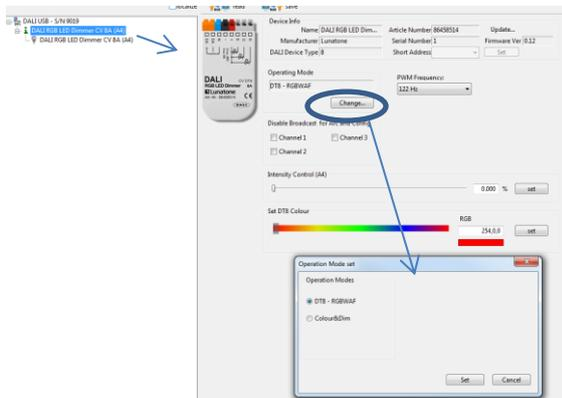
In addition, on the same page the PWM-frequency can be selected and basic control elements for testing each operating modes are available (slider for level and colour in the operating modes DT8 and Colour&Dim). Furthermore the broadcast control can be deactivated for each channel individually.
