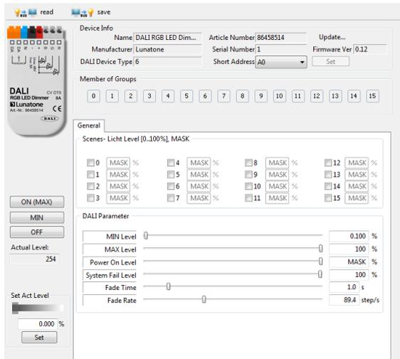
For each address the group membership can be set as well as scene values and DALI-parameters. In Colour&Dim operating mode, all values assigned to channel 2 are representing colours.
