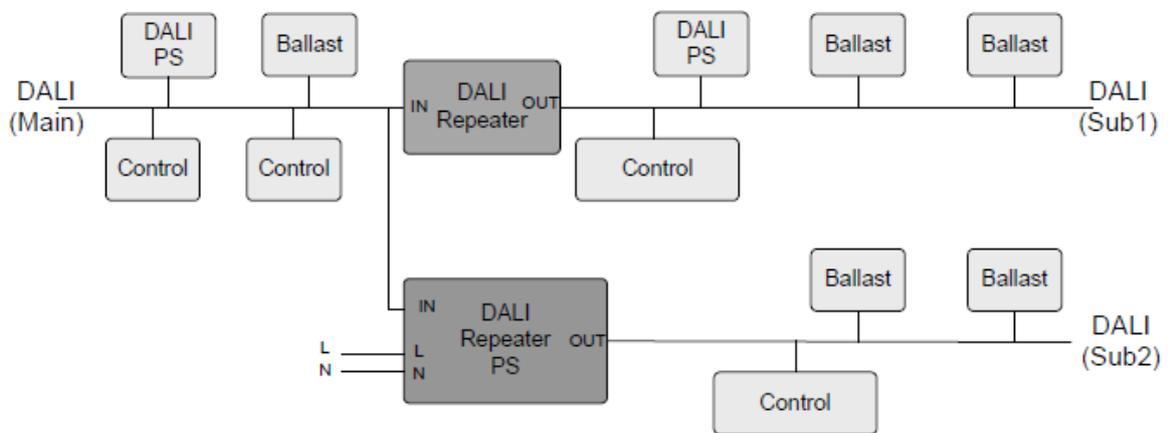
typical application: Dali commands from any control are transmitted in all DALI-lines, on the output of a DALI Repeater with integrated PS no DALI PS is needed
