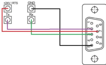
Connection diagram of a cable from RJ45 -> SubD (for direct connection to the RS232 of a PC, supply via RTS-Pin):
