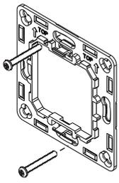
**Method 2:** Screw the bracket to the wall
